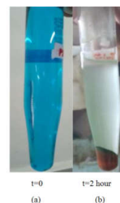
Fig 4 Adsorption test of the porous RF microspheres; (a) before adsorption (b) after adsorption
