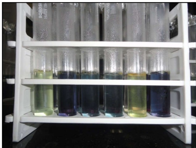
Figure 3 Dye extracted from the composite tooth interface into 65% nitric acid. The vials were then centrifuged at 14,000 rpm for 5 minutes after which dye absorption was measured by a semi- automatic spectrophotometer at 560 nm using concentrated nitric acid as a blank. (Figure 4)
