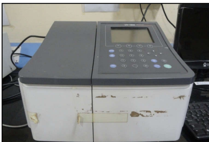
Figure 5 Spectrophotometer used for dye extraction method of microleakage detection. (SHIMADZU, Model No.UV- 1800)
