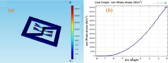
Figure 5 Von Mises Stress analysis of Design-II (a) 3D view and (b) line graph
