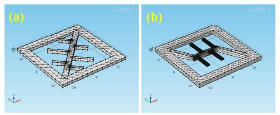
Figure 2 Meshing for Design-I (a) and Design-II (b)
