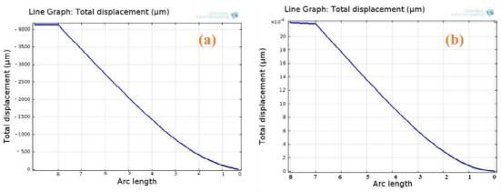
Figure 3 Total displacement of the microcantilever Design-I (a) and Design-II (b)
