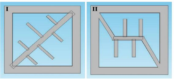
Figure 1 2D view of the proposed piezoelectric energy harvester Designs I & II.
