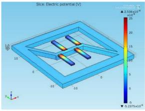
Figure 6 Potential generated in the microcantileverDesign-II
