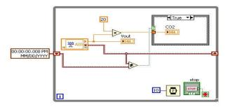
Fig. 6. Monitoring reading of GMM 221 CO2 sensor Data in LabVIEW.
