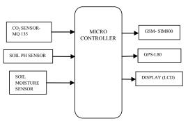
Fig. 2. The CO<sub>2</sub> sensor white grub detection system.
