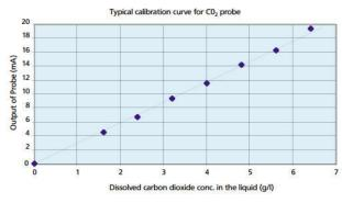
Fig 10 Typical linearized CO<sub>2</sub> response.
