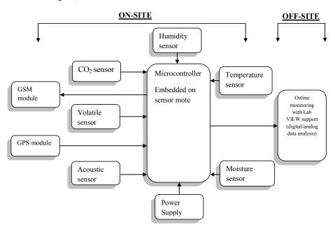
Fig. 5. The combine sensors system with LabVIEW support
