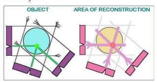
The "SkyScan-1072" is a compact desktop system for x-ray microscopy and microtomography. It consists of the combination of an x-ray shadow microscopic system and a computer with tomographic reconstruction software. This system allows making a non-destructive three-dimensional reconstruction of the object's inner structure from two-dimensional X-ray shadow projections.
