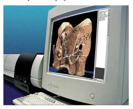
The equipment contains an x-ray microfocus tube with high-voltage power supply, a specimen stage with precision manipulator, two-dimensional x-ray CCD-camera connected to the frame-grabber and a Dual Pentium computer with colour monitor. However the 50% silver nitrate solution can cause erosion at margins giving confounding results.
