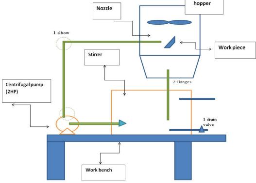
Fig.1 Schematic Diagram of Jet Tester
