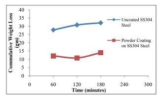
Figure 3 shows Variation in cumulative weight loss with respect to time at 45° impact angle at a flow rate of 2.5 litres/second.
