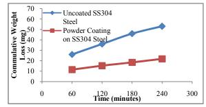
Figure 7 shows Variation in cumulative weight loss and time at a flow rate of 3.5 lit/sec.
