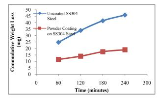
Figure 4 shows Variation in cumulative weight loss with respect to time at 60° impact angle at a flow rate of 2.5 Litres/second.
