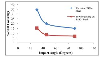
Figure 1 Shows variation in weight loss with respect to different impact angle at different flow rate.
