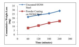
Figure 6 shows Variation in cumulative weight loss with respect to time at  $90^{\circ}$  impact angle at a 2.5 litres/second.
