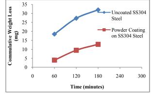
Figure 5 shows Variation in cumulative weight loss with respect to time at 75° impact angle at a flow rate of 2.5 Litres/second.
