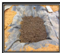
Figure 7 Treatment with Enretech-1, water, straw and uncontaminated soil
